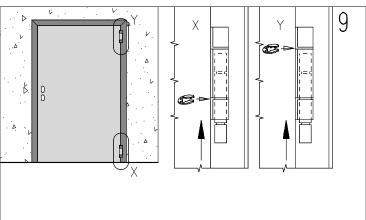
Apply the leaf by inserting the two pivots in the hinges and block them with the supplied retaining rings. Perform this operation very carefully.
