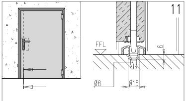
In case of Rever "Secur" door, plug the floor catho set to the floor.
