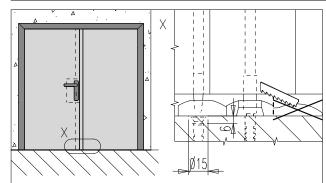
For SECUR-version doorset insert the application for the lower rod of the main leaf into the floor catch set and together with the floor catch set for the lower rod of the secondary leaf screw it on the floor; remove the two unneeded quides.
