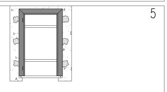
Shore up the doorframe opening and fix the frame—brackets with quick drying cement.
