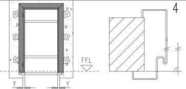
Fasten the door temporarily in the wall opening respecting the plumb—line, the FFL level and the parallelism to the wall.
