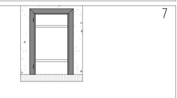
Remove the lower spacers in order to finish the floor.
