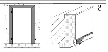
Remove the residual cement and the spacers, then proceed with the finishing and insert the rebate sealing into the groove of the doorframe.
