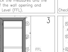
Bend up the frame—brackets and mark on the wall their positions respecting the FFL level. Create the apposite holes in the wall for the brackets.
