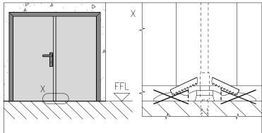
Use the same assembling procedure for the standard two leaved doors. Fasten with screw/plastic anchor and one drop of silicon the floor catch set for the lower rod of the secondary leaf and cut the four unneeded quides.
