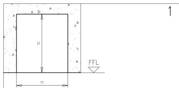
Unpack the doorframe, check the measures and the plumb line on both sides of the wall opening and establish the Finished Floor Level (FFL).
