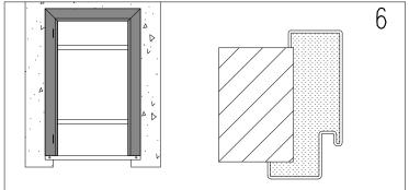
Fill up the space between the doorframe and the wall with mortar avoiding every deformation of the doorframe.
