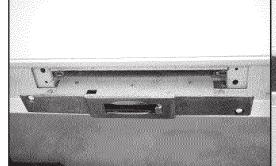
Insert the central lock with the hook drive turned look down. Make sure that the two rods will be coupled.
