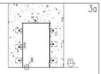
Bend up the frame—brackets and mark on the wall their positions respecting the FFL level. Create the holes in the wall for the brackets. Insert a spacer of 1 cm under the leaf of doors with wall opening L=1350 (X).
