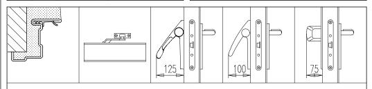
Optionals: rubber gasket — overhead doorcloser (the spring must be anyhow slightly loaded) — antipanic bar EXUS / TWIST and SLASH.
