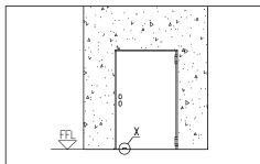
Fasten temporarily the door in the wall opening respecting the plumb—line, the FFL level and the parallelism to the wall. Insert a spacer of 1 cm under the leaf of doors with wall opening L=1350 (X).
