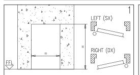
Unpack the door and verify the correspondence between the wall opening and the dimension printed on the coloured sticker applied on the frame. Establish the Finished Floor Level (FFL) and the opening direction.
