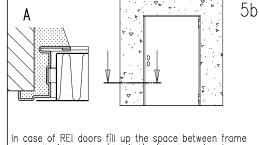
and wall with mortar (detail A) without curving frame.
