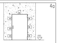
Fasten temporarily the door in the wall opening respecting the plumb-line, the FFL level and the parallelism to the wall.
