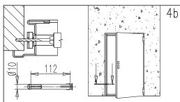
Open the door-leaf and fix the frame at presetted holes with expansion screws type Würth art. 0910436112 (expansion screws not supplied). Close again the door-leaf.
