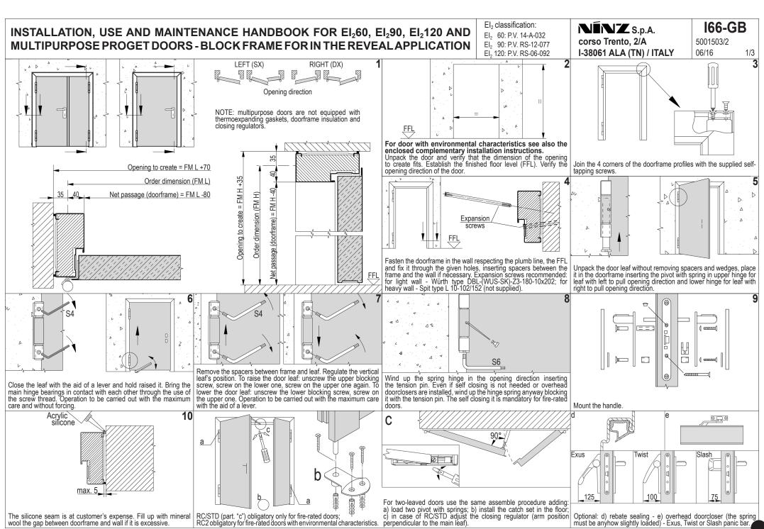
Optional: d) rebate sealing - e) overhead doorcloser (the spring must be anyhow slightly loaded) - Exus, Twist or Slash panic bar.
