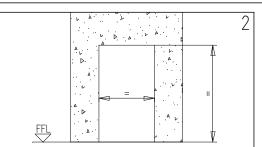
Unpack the door and verify that the structural opening corresponds with the dimension on the sticker. Fix the definitive Finished Floor (FFL) level and opening direction.
