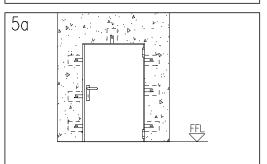
Bend up the frame-brackets and mark on the wall their positions respecting the FFL level. Create the
