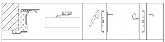
Optionals: rubber gasket — overhead doorcloser — antipanic bar TWIST — antipanic bar SLASH.
