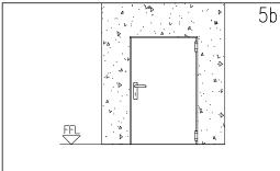
Fasten temporarily the door in the wall opening respecting the plumb—line, the FFL level and the parallelism to the wall.
