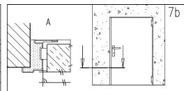
Fill up the space between frame and wall with mortar (detail A) without curving frame.
