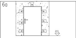
Fasten temporarily the door in the wall opening respecting the plumb—line, the FFL level and the parallelism to the wall.
