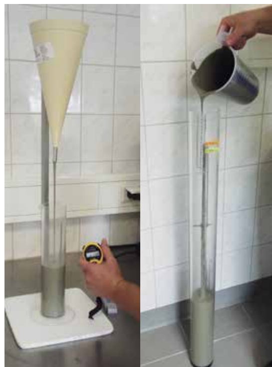
Determining the flowability, and the settling test with vertical tube (wick settling test)
