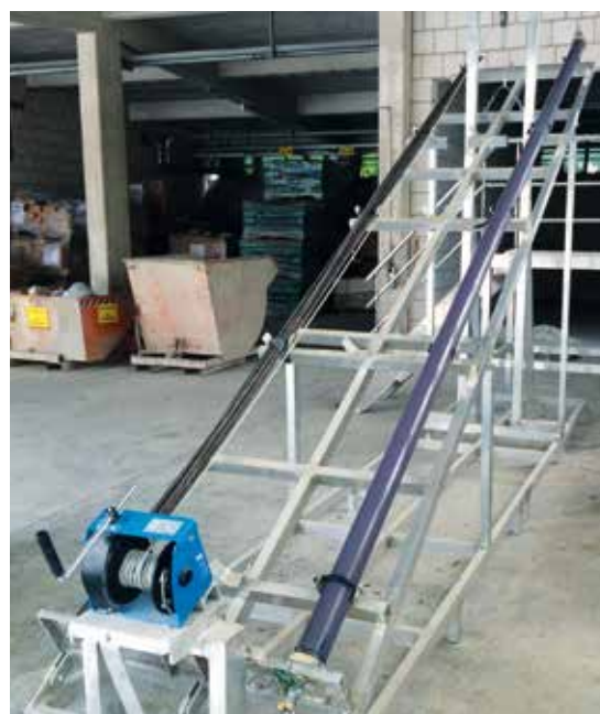
Settling test with inclined tube
